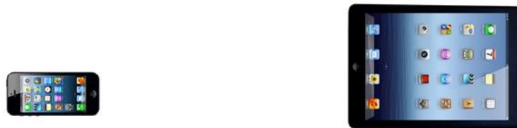
Figure 7: Experimental Blind Pepper's Ghost Configuration without Object. This is a view of the configuration from above. The iPhone (left) is spaced 31.7 centimeters from the iPad (right).
